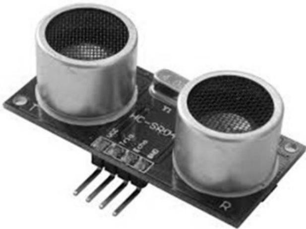
**Fig.2 : Ultrasonic Distance Sensor**
