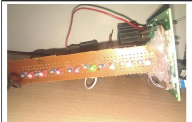
**Fig 5 : Prototype development board (Receiver) Front view**
